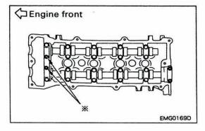
4. Install the camshaft brackets.
