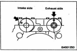
3. Install the camshaft brackets.
